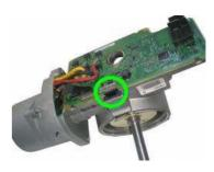
4) Use the appropriate welder to remove the "flat" connector.
