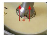
6) Pay attention at the new sensor. Spring clip has to be perfectly orthogonal at plastic structure, in order to make the sensor "disks" in-built.
