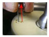
10) Reassemble hose, gasket and elastic ring.
