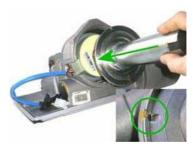
11) Insert the plug in its housing.
