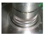
7) Before starting fitting process, the three reference signs must be perfectly aligned.
